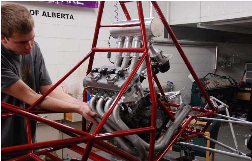
Dan Vaandrager fitting the exhaust.
